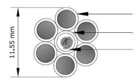
Aluminium Clad Steel Wire(35% IACS)
